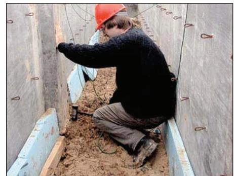
Performing SE/IR evaluation on concrete foundation walls
