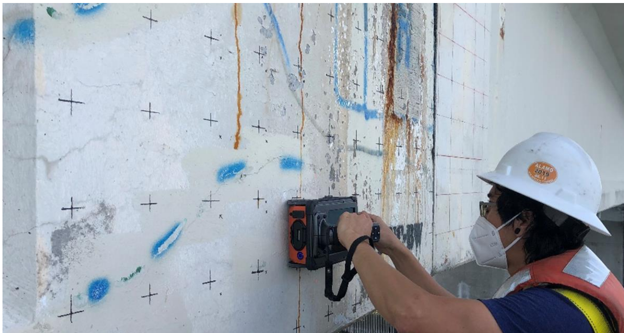
Figure 3: Horizontal GPR scanning on a 3 in (75 mm) grid (vertical scans were also completed) for 3-D GPR image
