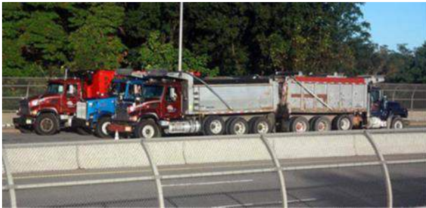
Figure 9. 6 loaded dump trucks – static test
