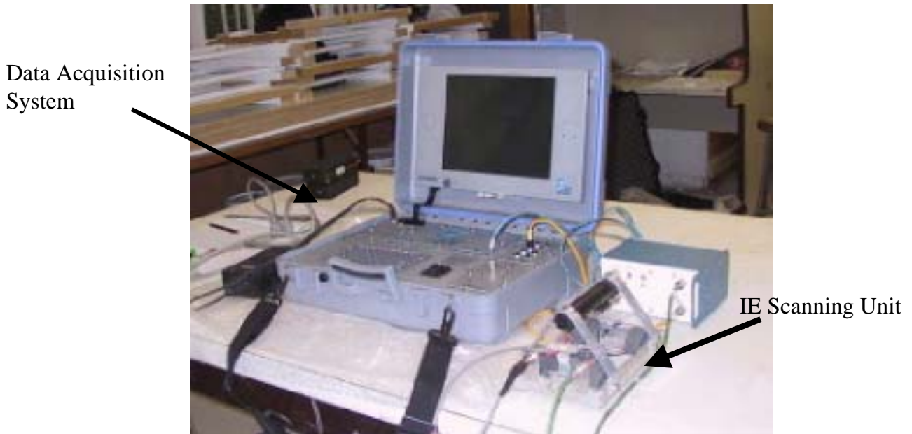
Fig. 2- IE- Scanning Unit with Data Acquisition
