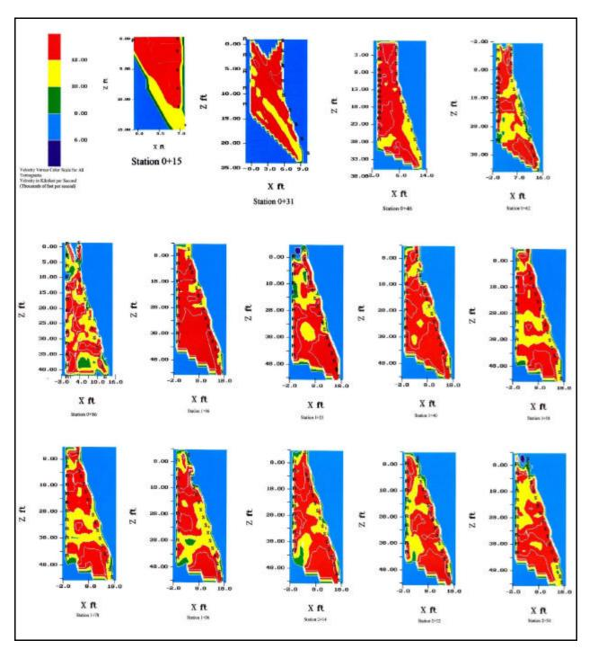
Figure 7. Tomograms for Stations 0+15 through 2+50
