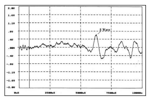
Figure 5. Example data trace showing low signal-to-noise ratio and no clear P-wave arrival. Note the strong S-wave arrival that was used in these instances.
